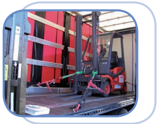
Fig.4 Example of Direct Lashing
