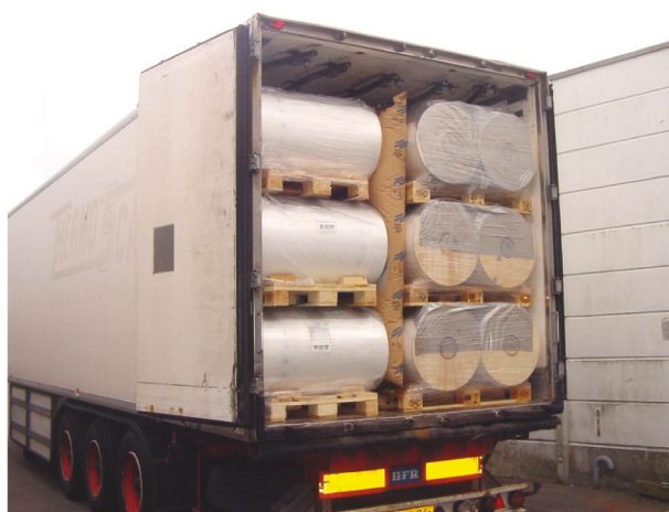
Figure 28 Filler between rows of cargo
