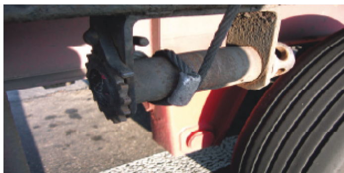
Figure 24: Steel wire rope tensioned by winch
