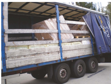
Figure 19: insufficient load securing by stretch wrap film only
