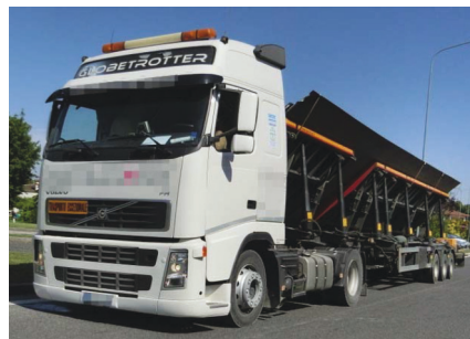
Figure 14: Steel plates transported under 45°
