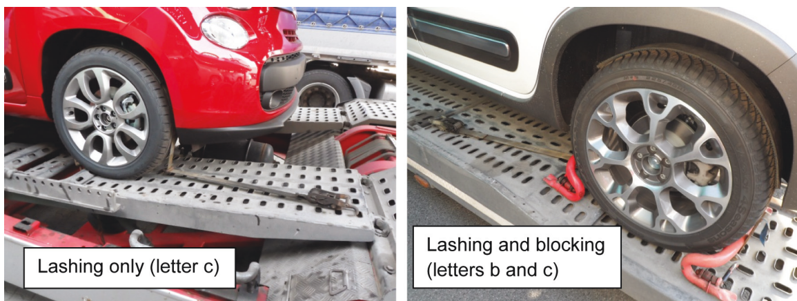
Figure 57: Securing arrangements for car transport
