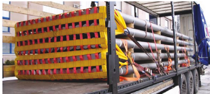
Figure 32: Securing with net and direct lashing in forward direction
