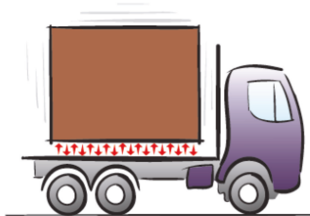
Figure 3: Vertical vibration during driving
