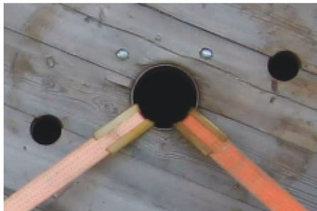
Figure 22: Protection at sharp edges
