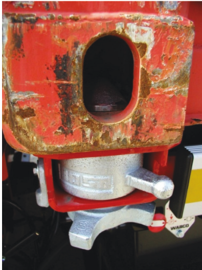
Figure 17: Twist lock with container
