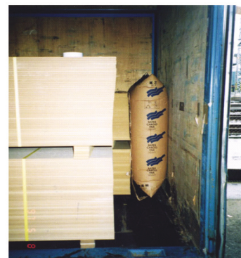
Figure 29: Air cushion for sideways blocking
