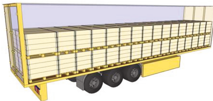
Figure 69: Stowing of pallets in XL coded vehicle
