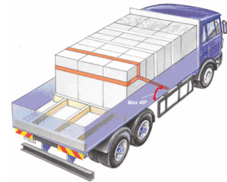
Figure 40: Spring lashing using a sling
