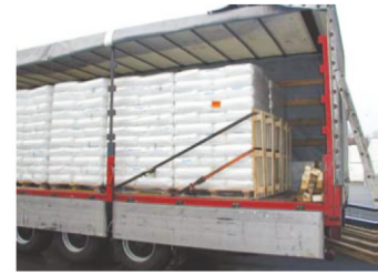
Figure 39: Spring lashing using pallets
