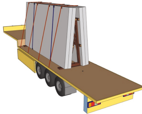
Figure 48: Securing with combination of blocking, A-frame, round lashing and top-over lashing
