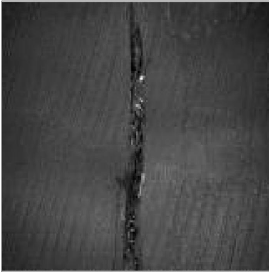
Fig. 14. This break resulted from a severe blow while overinflated.
