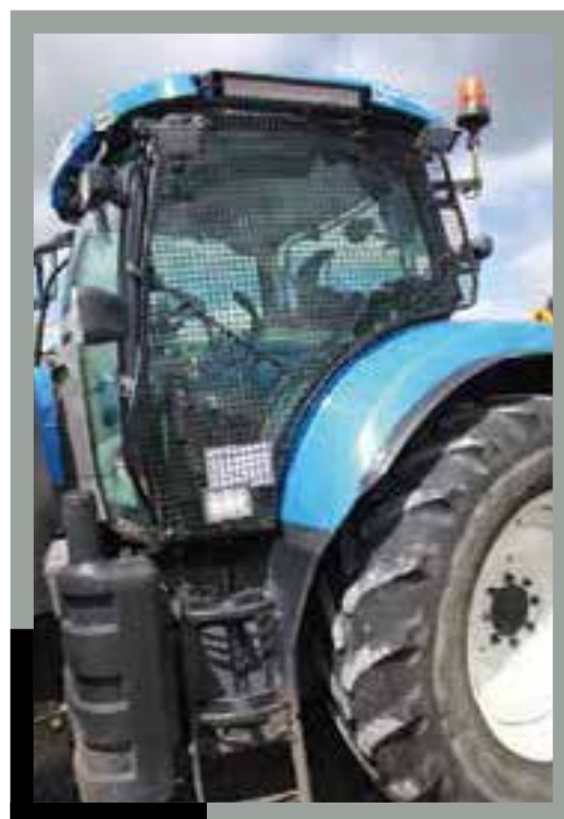
Install mesh on windows to protect from debris
