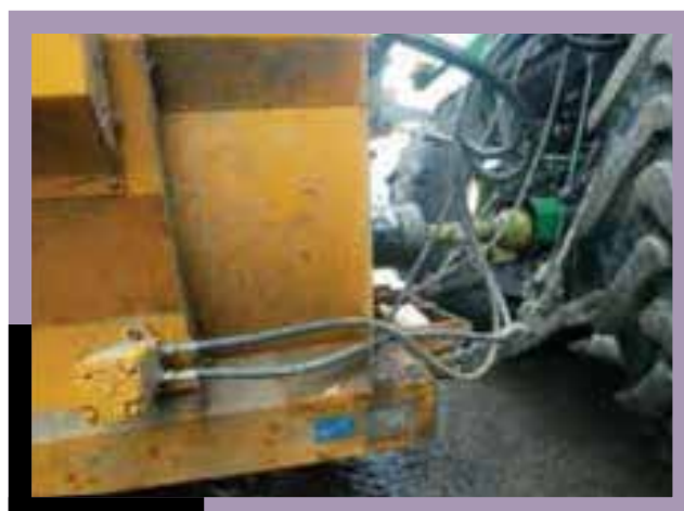
Keep PTO & hydraulic lines in good condition
