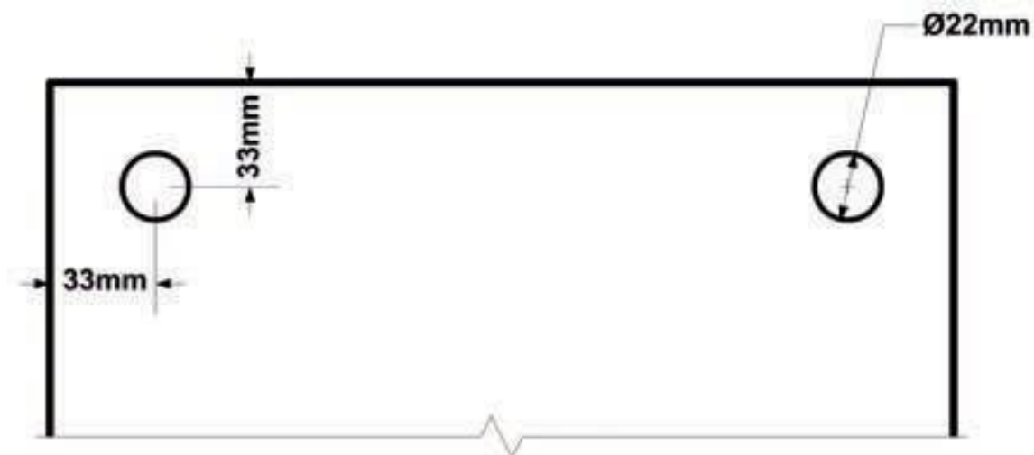
Steel baseplate with punched holes 20mm diameter anchors Maximum clearance hole = 22mm Minimum edge projection = 33mm
