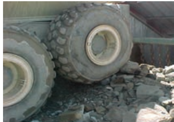
Figure 18: Unsafe tipping points
