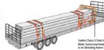
Figure 7. Example of correctly secured Precast Concrete load using chains
