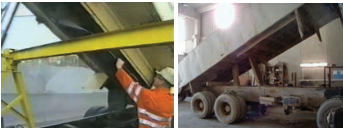
Two Acceptable Methods of Supporting a Tipper Truck Body During Maintenance Operations
