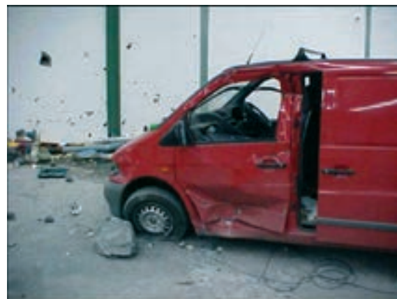
Figure 36: Damage caused by Fly-rock.
