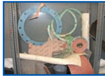
Compressed asbestos gaskets
