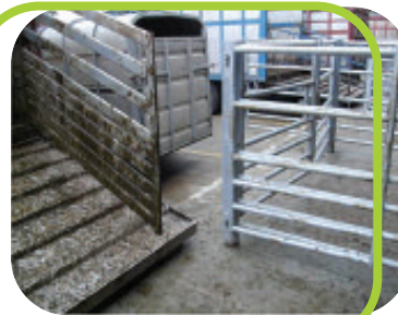
Position the trailer to avoid gaps like this
