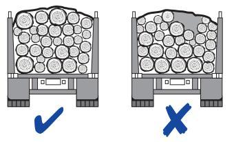
*Figure 10. Correct (left) and incorrect (right) loading of round timber*
