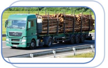
Figure 2. Example of a round timber vehicle equipped with headboard and stanchions
