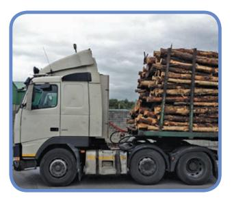
Figure 8. No headboard = no blocking capacity
