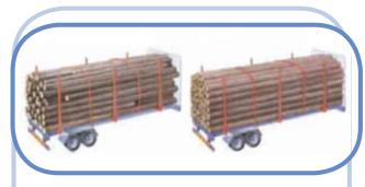
Figure 5. Load lashing should always be added vertically on round timber loads
