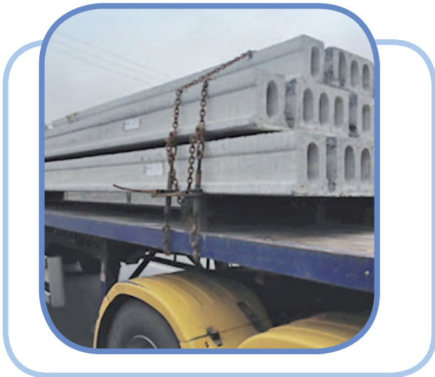
Figure 4. No Blocking Capacity
