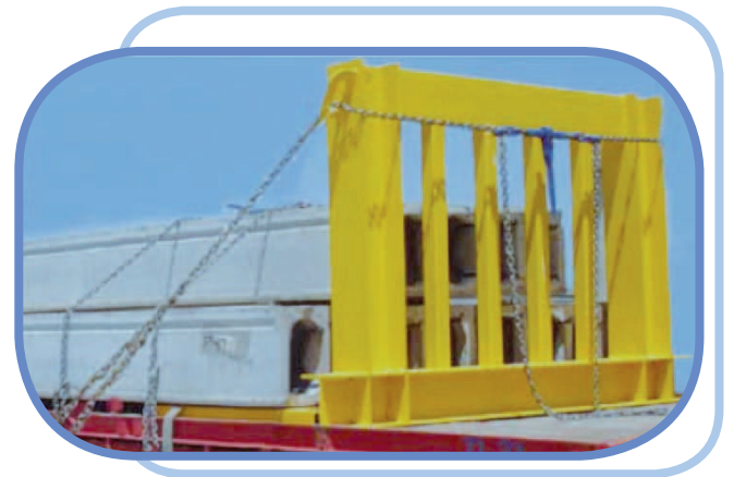
Figure 5. Example of moveable Blocking Frame to prevent forward movement
