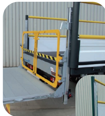
Typical example of column lift with runner mounted 3 position gates
