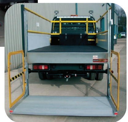
Typical example of column lift with runner mounted 3 position gates
