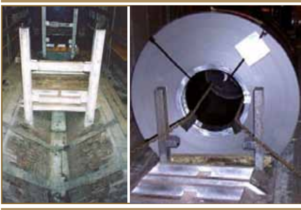
Fig. 81. Example of a (cross)beam for blocking of coils
