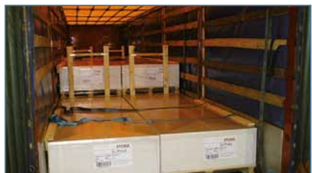
Fig. 19. Panel blocking of paper sheets on pallets
