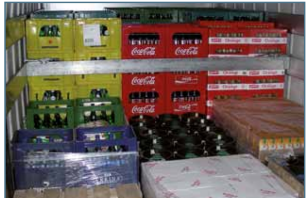
Fig. 13. Blocking by headboard and specially designed gates
