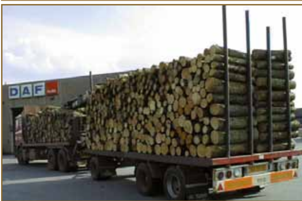
Fig. 69. Timber stacked transversely is not recommended!
