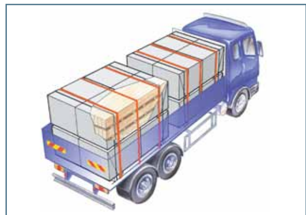
Fig. 51. Secured full load of sawn timber
