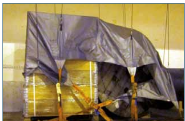
Fig. 42. Restraint system with integrated lashings
