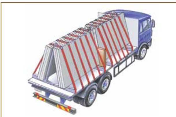
Fig. 63. Panels secured on a platform with blocking device in place
