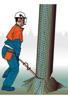
Figure 3: Use of breaking bar
