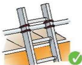
Figure 9 - ladder tied at top
