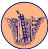
Workers must be able to get in and out of excavations safely. Generally, ladder access is used. Landing areas should be kept free of obstruction. All ladders must be secured to prevent slipping or sliding, and must allow for safe access and egress.
