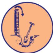
Before excavating, the adjacent area should be checked to ensure that the excavation work will not cause other structures to become unstable or collapse. Underpinning and propping may be required to stabilise such structures before excavation work begins.
