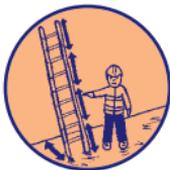
All ladders, including step ladders, must be: carefully selected for each task; carefully tied; of correct length; free from patent defects; set at the correct angle; and, where necessary, footed. Ladders must be controlled and checked frequently to ensure they are fit to use.
