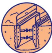
A Trench Box is a proprietary support system. Trench supports can be put in place without people having to enter the excavation. When it is in place, people can work safely inside the Trench Box.
