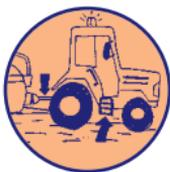
Agricultural tractors are often used on site. Where the power-take-off (PTO) shaft is used to transmit power to a towed accessory, the joining PTO shaft and its couplings must be fully guarded.
