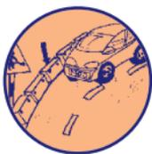
Where everyday transport moves close to road works, careful segregation must be planned, including the use of vehicle bollards, crash barriers, guardrails, signs, etc. The choice of the appropriate Vehicle Crash Barrier must be based on a Risk Assessment. This Risk Assessment should take into account the type and extent of work activity, including construction plant in use, duration of works, lines of sight, location, road surface, traffic speed, traffic volumes, width of road, etc.
