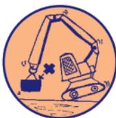
Lifting appliances and lifting gear should never be used to lift beyond their stated safe working load (SWL). This, as assessed by a competent person, is the maximum load that an item of lifting equipment may raise, lower or suspend under the particular service conditions.
