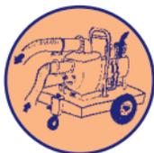
Water build-up in excavations should be removed with pumps to prevent flooding. Such pumps must be maintained in good working order, and be sited on firm ground at a safe distance from the crown of the excavation, so that they will not undermine the banks of the excavation or put the person operating the pump at risk from falling into the excavation.
