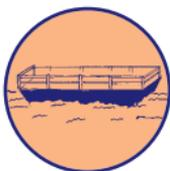
When work is taking place in or over water, a suitable working platform must be provided. Such platforms must be secured, be fully boarded, have edge protection and safe means of access and egress.
