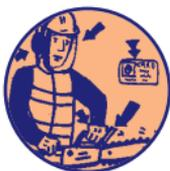
Chain saws must only be used by trained people. The saws must be regularly maintained and kept in good working order. The many safety features such as guards and chain brake should be checked before each use. All guards must be in place at all times. Appropriate PPE must be used.
