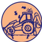
Operators must possess the appropriate training certification as prescribed in the Construction Regulations. The machine must be set up safely when digging: the hand parking brake must be engaged, direction levers must be in neutral, front bucket lowered, machine level, stabilizers dropped appropriately to the ground and all wheels must be off the ground.
