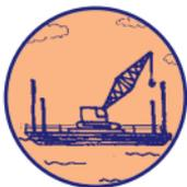
A pontoon is a floating vessel, usually flat-bottomed, used as a working platform on water. All plant and equipment carried on pontoons must be adequately secured, to prevent inadvertent movement. A crane should have its tracks securely lashed with chains or equivalent. At the end of a shift the crane's jib should be dropped and lashed. As a working platform it must be completed with edge protection and adequate welfare facilities, etc.
