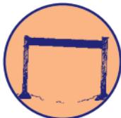
Suitable barriers should be placed around excavations when work is in progress; typically, the barrier should be set and secured a safe distance from the crown (leading edge) of the excavation, e.g. 2 metres (decided on by a competent person). At the end of each day, these barriers should completely surround the excavation and be strong and high enough to prevent people falling into the excavation.
