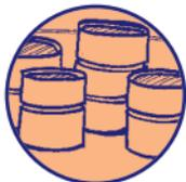
Pipes and other materials should be stacked in a safe manner, with wedges, to prevent pipes and other materials from falling or rolling on to people. Large circular sections (such as manhole sections) should be stored on the flat and not on their circular sides.
