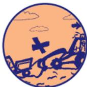
If any vehicle gets into difficulty on site, back actors, excavator booms, lifting arms, etc, should not be used to pull the vehicle free (unless this might prevent injury or death). Only appropriate plant should be used to rescue vehicles, and it should be done from an approved towing point.
