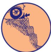
A chock or a stop block is a block (e.g. sleeper) that prevents a vehicle from approaching too close to the side of an excavation, which otherwise could cause the sides of the excavation to collapse or itself roll into the excavation.
