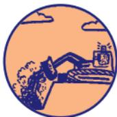
Back Filling is the re-instatement and making safe of the excavation. It must be carried out immediately after the support systems are removed. Stop blocks should be used to alert drivers of vehicles (dumpers, lorries, teleporters, etc) when they are approaching the side of the excavation.
