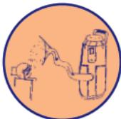
Tools and equipment which generate dust or fume clouds should be fitted with appropriate extraction and/or wetting aids.
