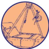
A tripod is a standard piece of rescue equipment for people working in confined space. With a tripod, a person can be lowered into the confined space by a 'buddy' and, more importantly, be raised out of it.
