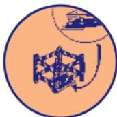
Generally in combination with barriers, covers (e.g. steel plates) should be placed over excavations. These should be appropriately secured and strong enough to prevent persons from falling through.
