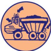
All dumper trucks should possess side mirrors, flashing beacons and audible reversing alarms. Most articulated dumpers will require CCTV to the rear.
