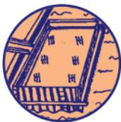
A cofferdam is a temporary dam formed using sheet piles, which enables construction on the dry side below water level. For work below 10 metres a caisson may be needed. Detailed method statements and risk assessments must be prepared and communicated to all workers involved.
