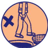
All ground openings, manhole openings, etc, as soon as they are created, must be guarded to prevent falls. Usually the opening is surrounded with visible guard rails and toe-boards that are anchored and fixed securely. Where openings are covered, the covers (e.g. manhole covers) must be of adequate strength
