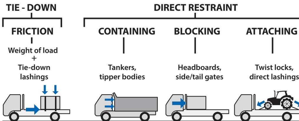
Figure 3. Load restraint methods (To control forward + rearward motion)
