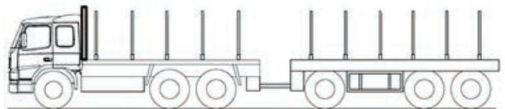
Figure 2. Example of a round timber vehicle equipped with headboard and stanchions
