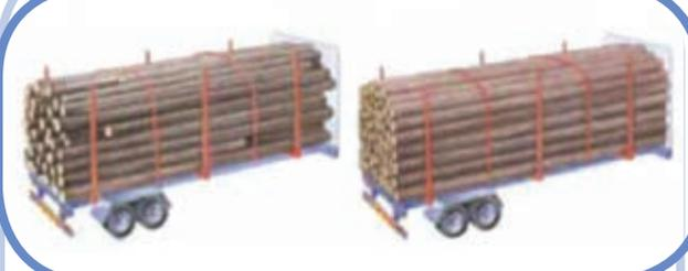
Figure 5. Load lashing should always be added vertically on round timber loads
