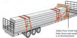
Figure 1: Example of correctly secured Precast Concrete load using chains.
