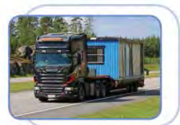
Figure 1. Prefabricated building transport
