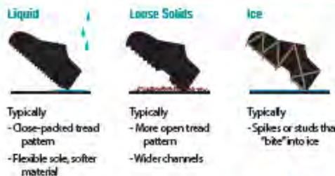
Figure 3. Typical sole properties of slip-resistant footwear by contaminant
