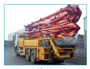
Fig 3: Truck Mounted Concrete Pump with Boom and Pipeline
