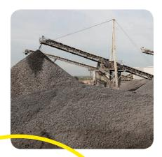
Simultaneous tipping and extraction to and from a stockpile should never be carried out as it can lead to instability.
