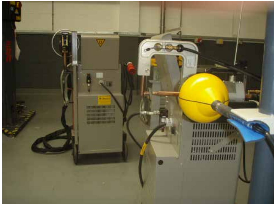
Figure 6.7 — Measurements around the repair shop spot welder fitted with a ‘C-type’ gun and the 160 mm arm installed. The ‘X-type’ gun welder is in the background
