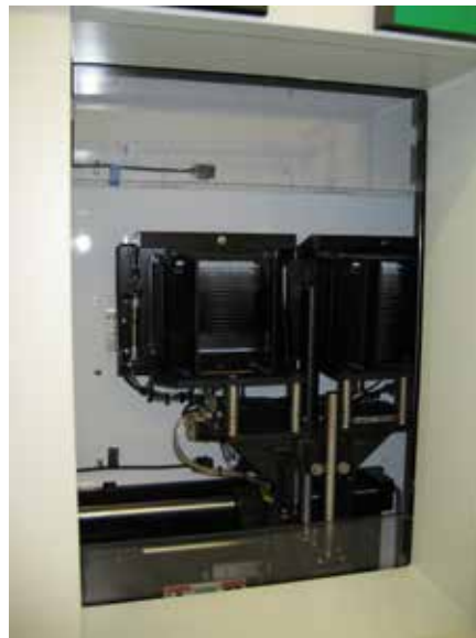
Figure 9.1 — Wafer loading area
