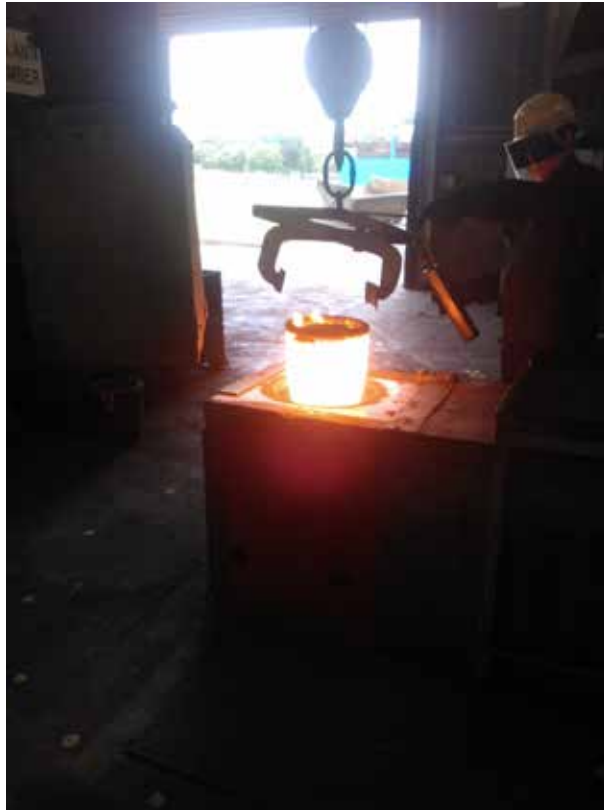
Figure 8.5 — Tasks involving close access to the furnace were performed with the furnace switched off
