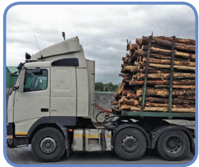
Figure 8. No headboard = no blocking capacity
