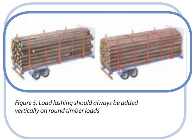
Figure 5. Load lashing should always be added vertically on round timber loads
