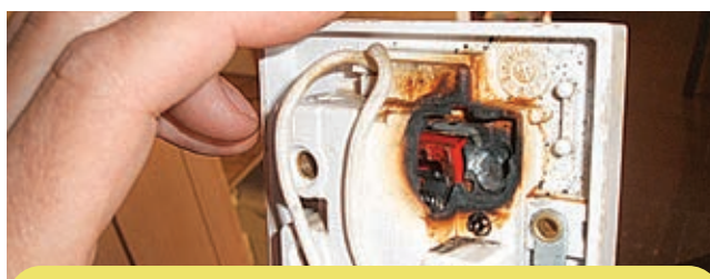
Fig 7.3 Potential ignition source from electrical equipment
