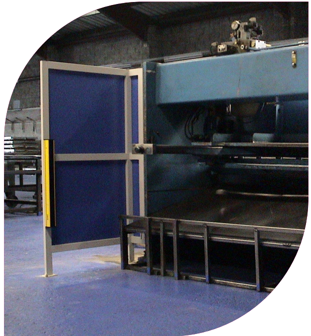
Light Guard at the rear of the guillotine machine.
